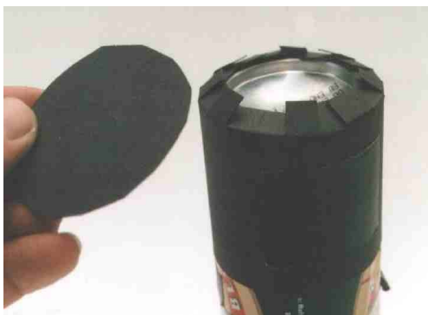
Making a light proof lid out of card. (This is covered with black gaffer tape after the photographic paper is inserted)
