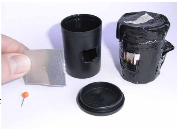
35mm Film Pot camera. Notice hole cut in plastic tub and final taped up version. A pencil has been taped on the back to point it upwards to catch the height of the summer sun.
